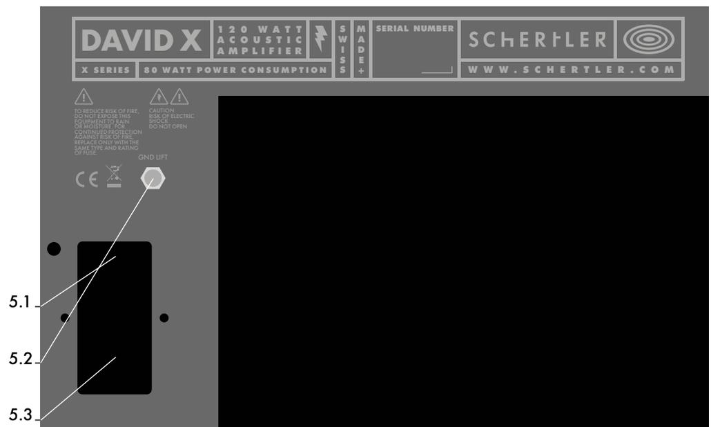
5.1. POWER ON/OFF: System ON/OFF switch.
