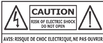
On a product, a lightning flash within a triangle indicates the presence of uninsulated “dangerous voltage” within the product enclosure. This may be of sufficient magnitude to cause risk of electric shock.
