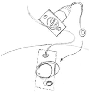
4. Thread the string in your hand through the screw hole of the XLR connector. Slip the transducer inside the instrument and fit the connector into the hole.
