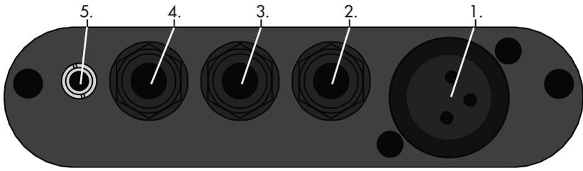
1. MIC IN: This enables the connection of a condenser microphone or a dynamic microphone (if necessary, press the PHANT button to power the microphone).
