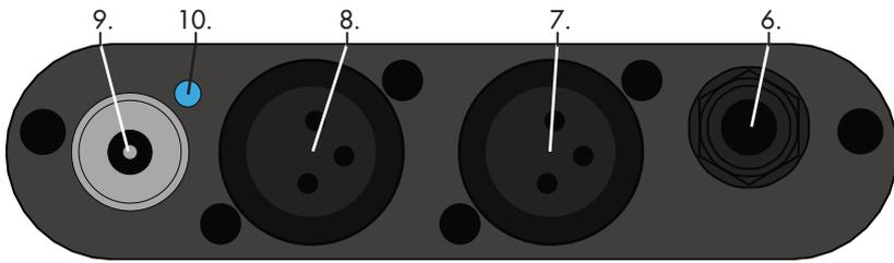
6. MASTER OUT UNBALANCED: The signal can be sent to an active loudspeaker or/and to another device. Output volume depends on both the VOLUME and MASTER VOLUME control: use the latter to only adjust the volume being sent to the speakers while leaving the other settings unchanged.
