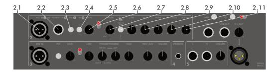
2.1. MIC INPUT (XLR): This input is electronically balanced for XLR-type connections. The channel is designed for any kind of microphone source e.g. dynamic and condenser mics.
