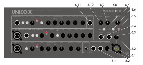
5.1. FX RETURN: Left and Right unbalanced jack socket for the return of external effects. This can also be used as a 5th input channel to accommodate an extra line level device.
