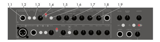
1.1. INSTRUMENT IN: An unbalanced input for the connection of 1/4'' jacks, with optimal sensitivity for high level signals. The electronics will adapt to any situation - no special action is required.
