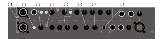
3.1. MIC INPUT (XLR): This input is electronically balanced for XLR-type connections. The channel is designed for any kind of microphone source e.g. dynamic and condenser mics.
