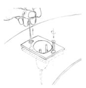
5. Pull the string towards you and put the metric screw into the free hole. Fix the screw with your screwdriver.
