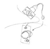
4. Thread the string in your hand through the screw hole of the XLR connector. Slip the transducer inside the instrument and fit the connector into the hole.
