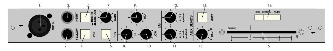
1. MIC IN: This XLR input can receive balanced signals from -50dBu to -7dBu (a range of 43dB). Intended as a dedicated microphone input, the wider dynamic range effectively enables any audio signal to be connected.
