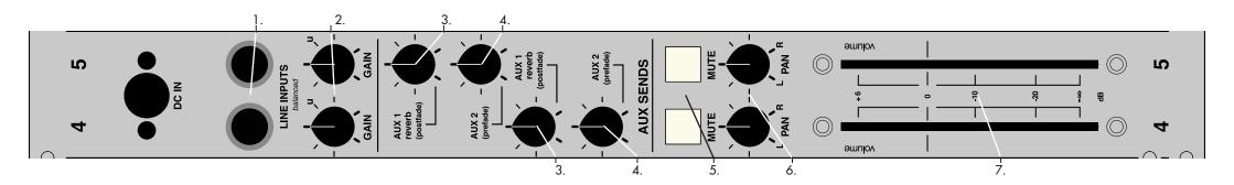
The "stereo" line channel effectively consists of two independent mono channels, each with their own controls. It can either be used as a stereo input or as 2 x mono inputs.
