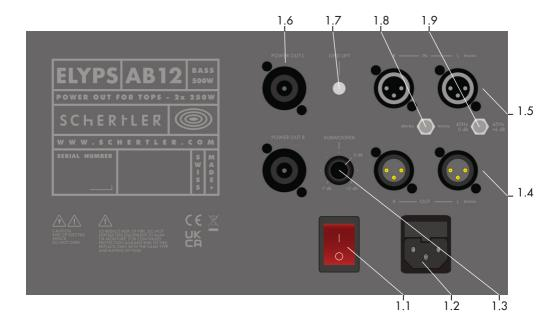
1.1 POWER ON/OFF: System ON/OFF switch
