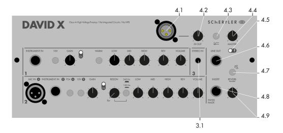
3.1. STEREO IN: 1/8" mini jack stereo input for PC, MP3 and other electronic devices. Volume depends on the MASTER volume regulation.
