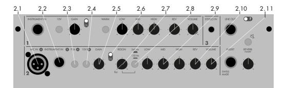
2.1. MIC INPUT (XLR): This input is electronically balanced for XLR-type connections. The channel is designed for any kind of microphone source e.g. dynamic and condenser mics.
